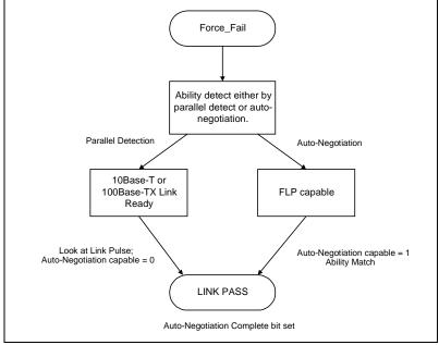
Figure 10. Auto-Negotiation and Parallel Detect
